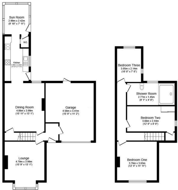
Ground Floor Floor area 88.0 sq.m. (947 sq.ft.) First Floor Floor area 57.8 sq.m. (622 sq.ft.)
